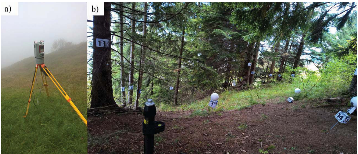
Fig. 3. (a) The scanner Riegler VZ-2000. (b) Field measurement. The white spheres are used for co-registration of seven scans.
